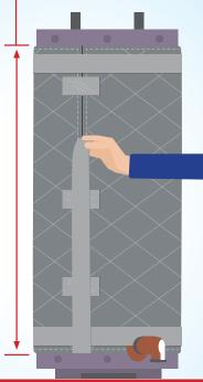
Safety Note: Don't set the thermostat above 130°F on the electric water heater with an insulating jacket or blanket - the wiring may overheat.
