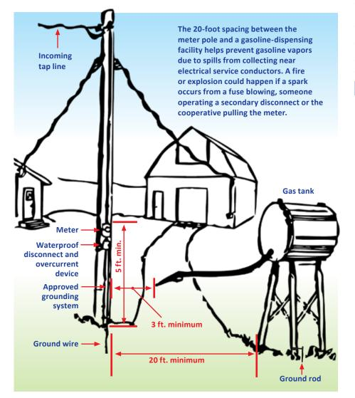
For Access Energy Cooperative to change the location of existing meter poles would be quite costly. Therefore, we ask members to check to make sure their gasoline dispensing facilities are located 20 feet from the meter pole. The end of the dispensing nozzle should not be within 3 feet of the meter pole.
