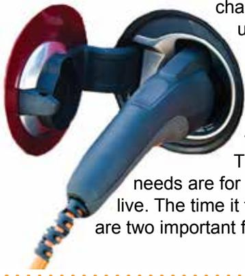
common home refueling unit, known as a Level 1 charger, is also considered the slowest. For example, it could take anywhere from five to 100 hours for an electric car to completely recharge when it is hooked up to a 120-volt household outlet. The advantage, though, is that this type of unit is low cost and easy to use.
